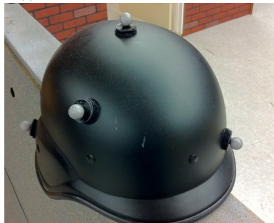
Figure 3: A helmet with retroreflective markers
