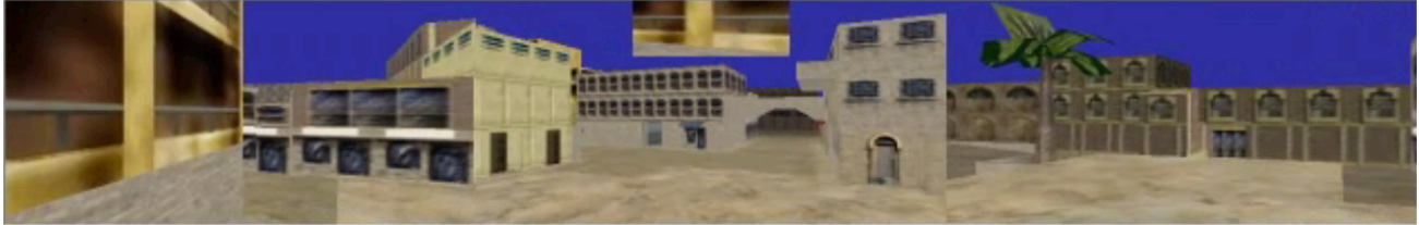
Figure 1: Example layouts created using the texture approach. The "bow tie" layout has a FOV of 225 degrees with five 45-degree cameras. The "rear view mirror" layout has 270 FOV (three 90-degree cameras) in its primary view, with a fourth 90-degree camera inset at top center with normal reversed as a rear-view mirror.
